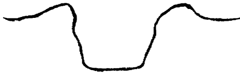
2 SHAPE EXCAVATION WITH SHOVELS TO FIT BUNKER
